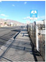
Obstructions and uneven sidewalk surfaces along East Central Ave. Fencing on the outside edge the sidewalk limits the usable area and forces pedestrians to walk closer to the roadway edge.
